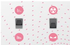
This will calibrate the module to 0V at the TIME CV input. Before powering on the module, make sure the TIME CV input is unpatched. The HOLD and OVERLOAD LEDs will flash three times to indicate that the module has been calibrated. Your module has already been calibrated so there is generally no need for you to do this.
